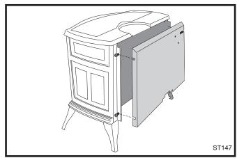
Fig. 16 Remove rear shroud.
