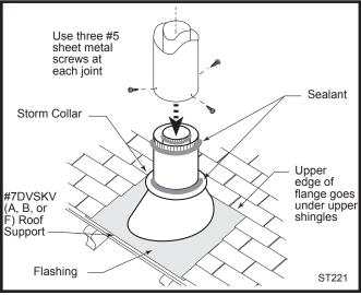
Fig. 33 Roof support and flashing.
