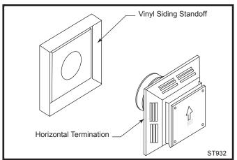
Fig. 43 Vinyl siding standoff and horizontal termination.
