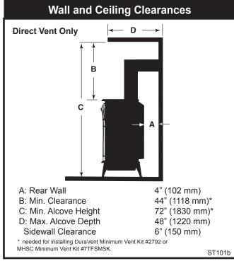
Fig. 6 Dimensions and clearances to ceiling or alcove.
