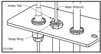
Fig. 69 Remove pilot orifice.
