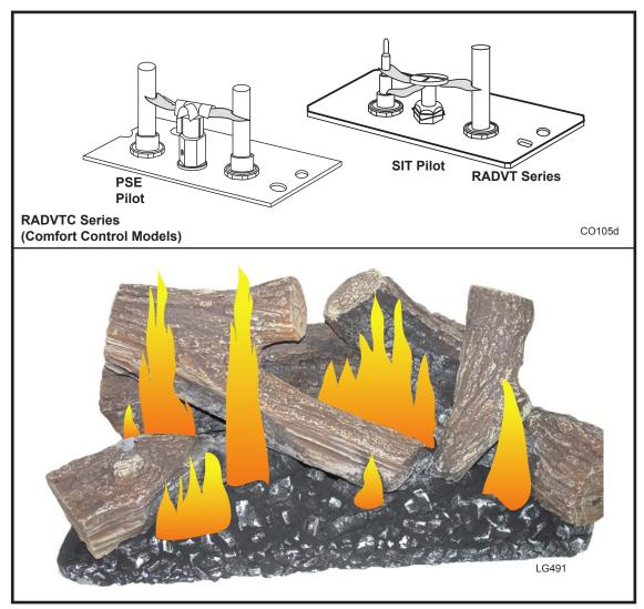
Fig. 56 Correct pilot and burner flame appearance.
