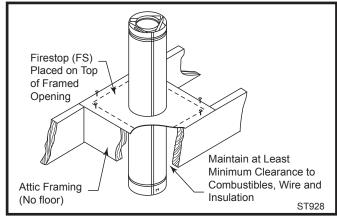
Fig. 39 Firestop spacer.
