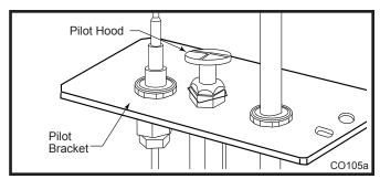
Fig. 68 Remove pilot hood.
