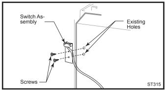
Fig. 52 Attach switch assembly to rear shroud.
