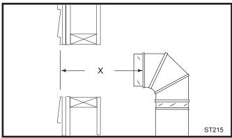
Fig. 27 Measure the horizontal length.
