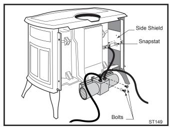
Fig. 17 Attach blower assembly and snapstat.
