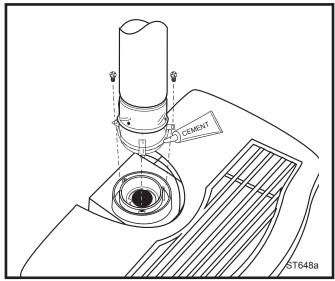
Fig. 20 Attach inner assembly to flue collar.
