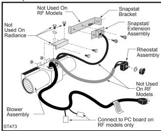
Fig. 15 Fan kit components.
