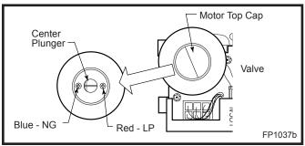
Fig. 66 Depress and turn center plunger.
