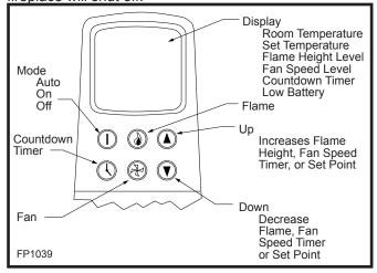
Fig. 58 Transmitter diagram.
