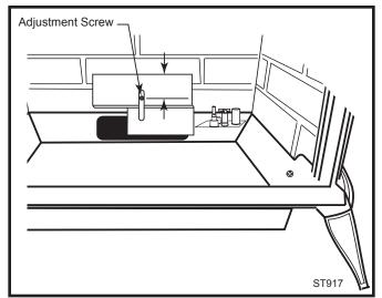
Fig. 9 Loosen screw to adjust restrictor plate.
