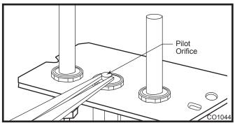
Fig. 71 Remove pilot orifice.
