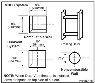
Fig. 24 Locate vent opening.
