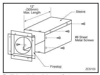
Fig. 25 Assemble the wall sleeve and firestop.
