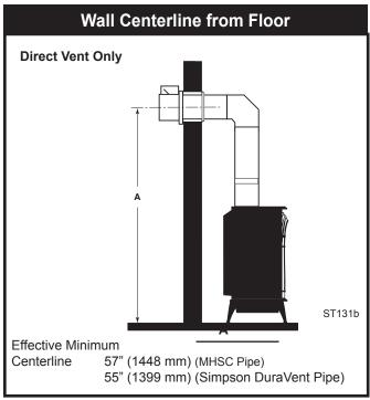
Fig. 5 Minimum wall centerline.
