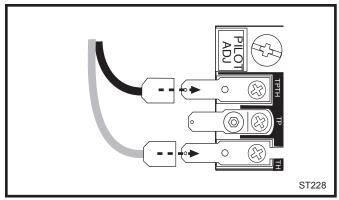
Fig. 53 Attach switch wires to valve.
