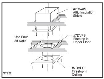
Fig. 32 Install firestops and attic insulation shield.
