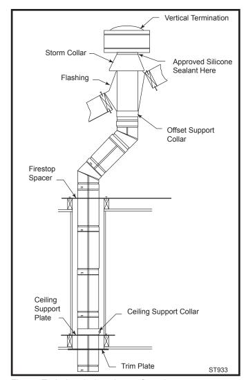
Fig. 44 Typical vertical venting configuration.
