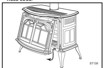
Fig. 46 Remove the stove front.
