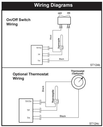
Fig. 80 On/off switch and optional thermostat circuit.
