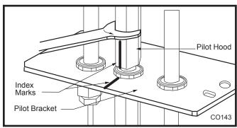
Fig. 70 Remove pilot hood. (Your pilot may have a different appearance.)
