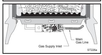
Fig. 60 Attach the gas line to the right side of the valve.
