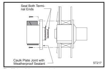
Fig. 29 Install the vent terminal.
