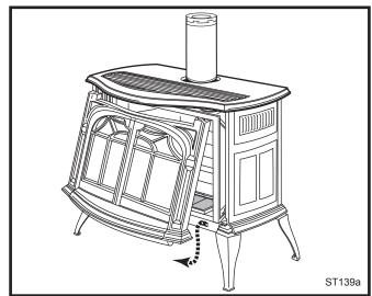
Fig. 76 Remove the Stove Front.
