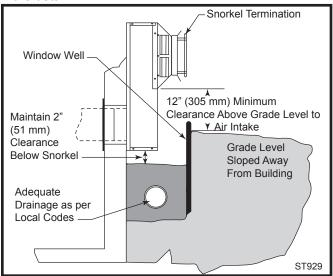
Fig. 40 Below grade installation.
