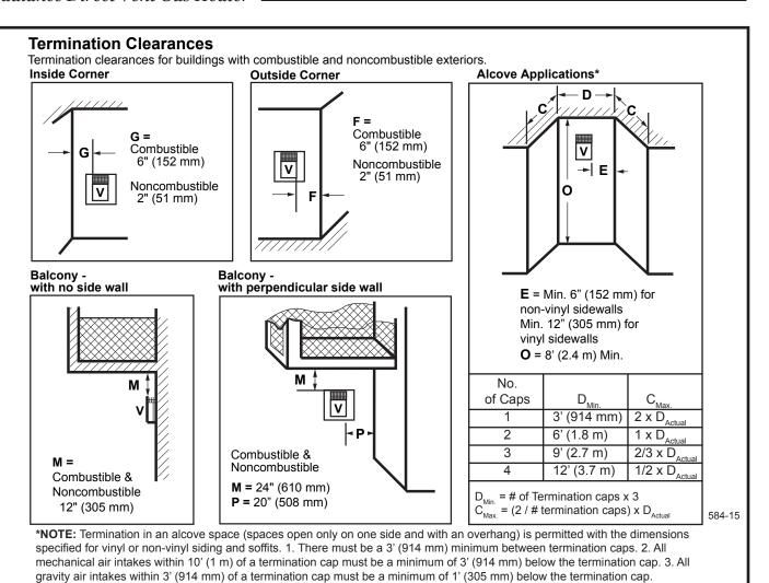
Fig. 12 Termination clearances.
