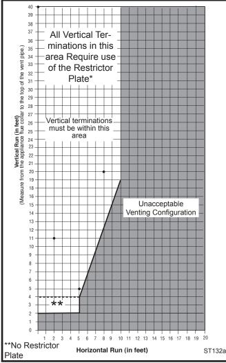
Fig. 8 Vertical vent termination window.
