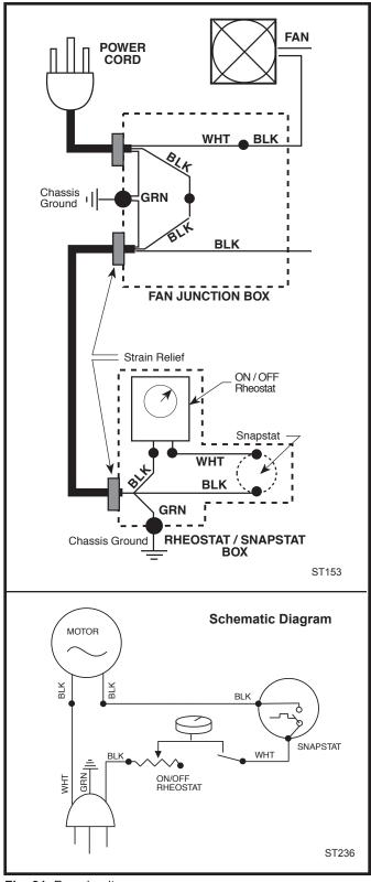
Fig. 81 Fan circuit.
