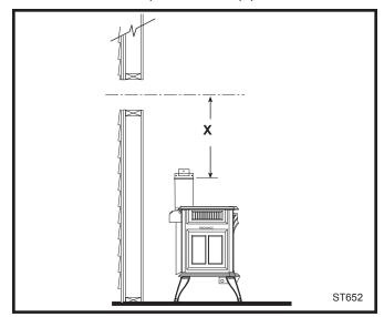
Fig. 26 Determine the vertical pipe length.
