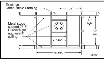
Fig. 23 Reflected ceiling plan.
