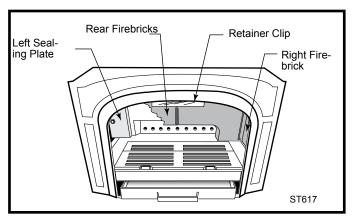
Fig. 33 Remove left and right sealing plates.
