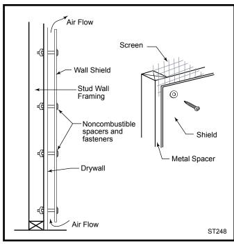
Fig. 13 Approved wall shield construction.
