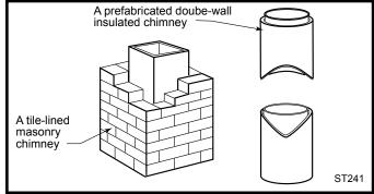
Fig. 3 Standard chimney types.
