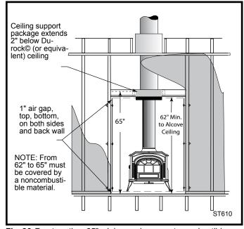
**Fig. 26** Front section: 65" minimum clearance to combustibles on front face. Combustible facing may overlap metal studs by <u>only</u> 1". It should not extend below the height of the noncombustible ceiling.
