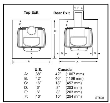
Fig. 11 Required floor protector dimensions.
