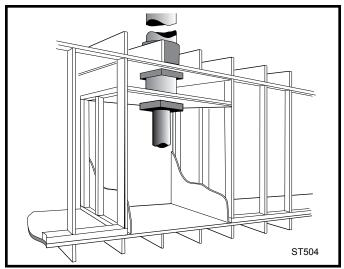
Fig. 22 Cutaway perspective of alcove installation.
