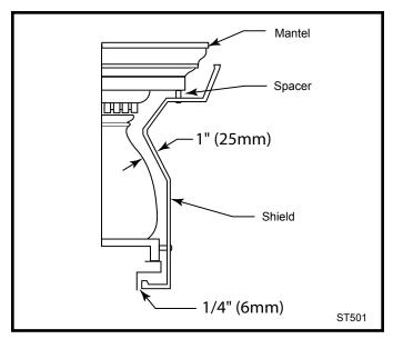
Fig. 14 A custom-formed mantel shield.
