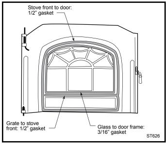
**Fig. 39** Two different gasekt sizes are used to seal the front door.
