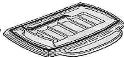
FIG. 5 CEMENT CHANNELS IN BOTTOM
