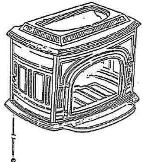
FIG. 9 REPLACE TIE RODS
