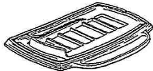
FIG. 5 CEMENT CHANNELS IN BOTTOM
