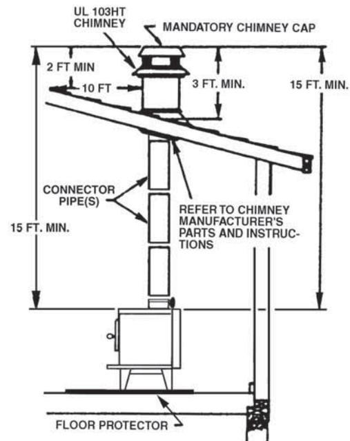
Fig. 12 - Chimney Construction Through Roof
