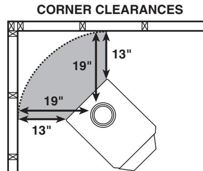
**Fig. 6 – Minimum Corner Clearance Dimension from Combustible Surfaces**
