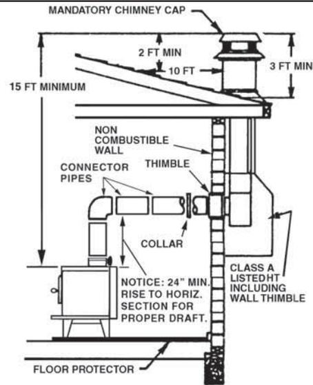
**Figure 13 - Chimney Connection to Firebox through Masonry Wall**
