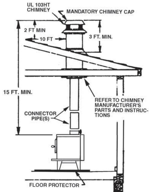
Fig. 11 - Chimney Construction Through Attic Space
