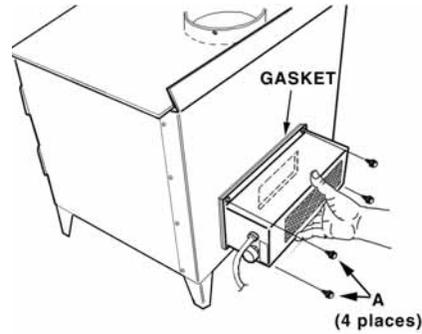
**Fig. 4 – Blower attaches to rear heat deflector**
