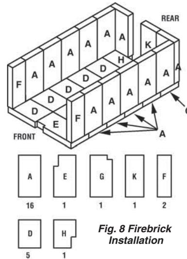
**Fig. 8 Firebrick Installation**
