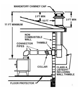
Fig. 14 - Chimney Connection to Firebox Through Masonry Wall
