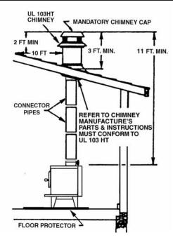
Fig. 13 - Chimney Construction Through Roof
