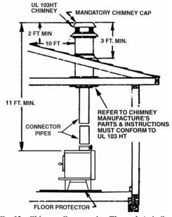
Fig. 12 - Chimney Construction Through Attic Space
