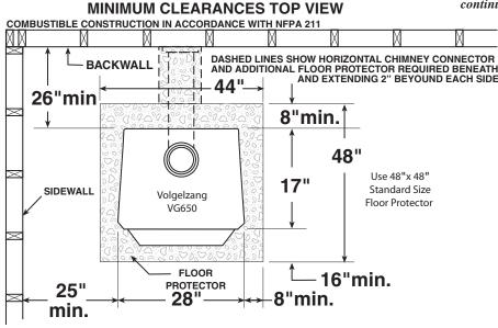
Fig. 7 – TOP VIEW Minimum Clearance Dimensions from Combustible Surfaces
