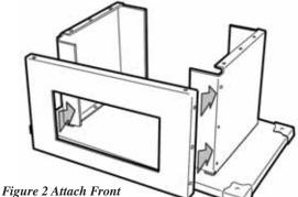
Figure 2 Attach Front Panel to Side Panels.
