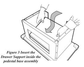
5. Insert the pedestal drawer support (#16) into the pedestal assembly. Secure with two (2) sheet metal screws from the back of the assembly.
