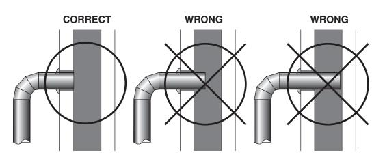
Fig. 10 – Stovepipe/Flue Connections
