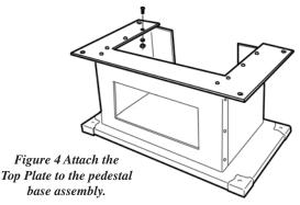
6. Attach the top plate to the pedestal assembly, figure 4, with machine screws, lockwashers and hex nuts.
