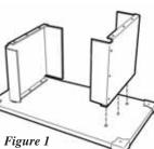
4. Attach the front panel (#17) of the pedestal base assembly to the sides. Notice: the front panel fits *over* the sides, figure 2. Attach the front panel to the side panels with machine screws, lockwashers and hex nuts (three each side).
