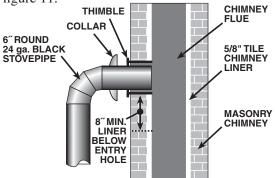
Fig. 11 - Masonry Chimney Connection
