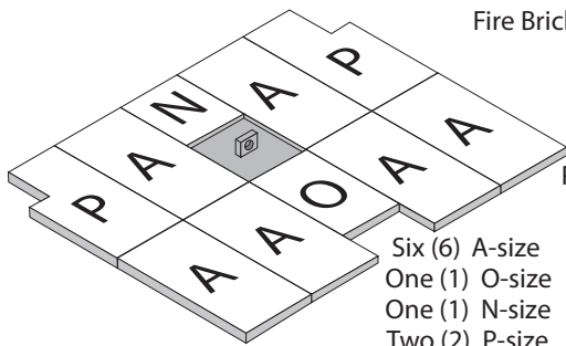
Figure 13a – Step 1, Bottom Firebrick Arrangement
